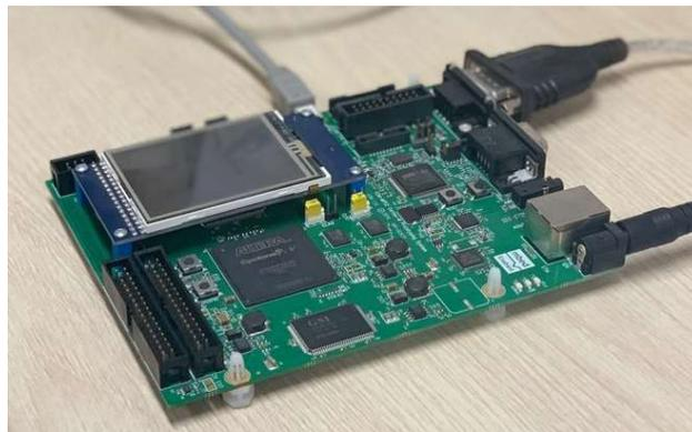
[ ARM MPS2+FPGA Prototyping Board ]
