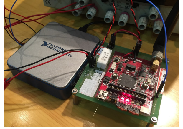
Fig. 8. The DAQ hardware (on the left) and the sensor device (on the right).
