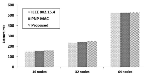
**Fig. 9** CE traffic (BO=SO=3): The highest priority to emergent traffics in the proposed scheme results in the highest latency of the proposed scheme.
