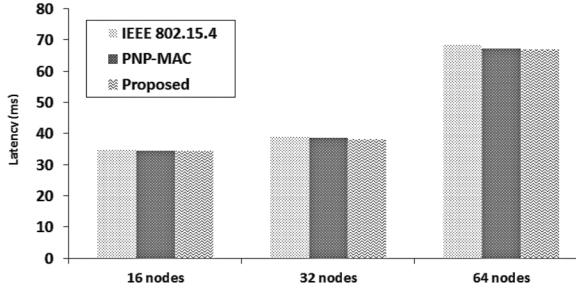
**Fig. 7** Medical traffic (BO=SO=3): Due to priority-based CTS, the proposed scheme and PNP-MAC shows a little lower latency than IEEE 802.15.4.
