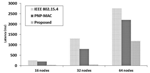
**Fig. 5** Emergent traffic (BO=4/SO=3): Due to both MP and EP, the proposed scheme outperforms IEEE 802.15.4 and PNP-MAC in terms of emergency handling.
