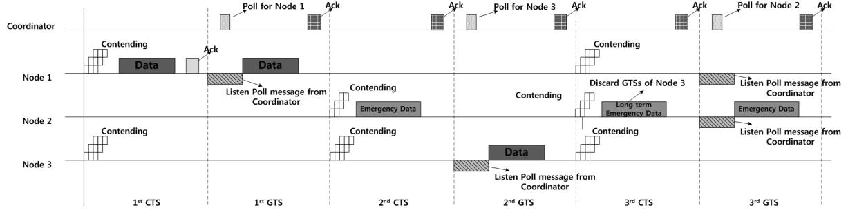
**Fig. 2** An example of emergency handling mechanism on MP.
