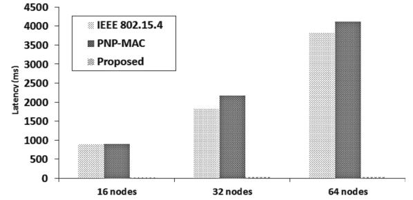
**Fig. 6** CE traffics (BO=4/SO=3): Due to the additional CAP in EP, the proposed scheme lowers the latency of CE traffics dramatically.
