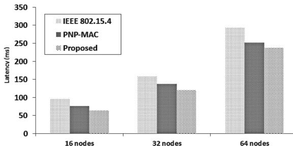
**Fig. 8** Emergent traffic (BO=SO=3): With the help of MP, the proposed scheme provides the lowest latency even in case of BO=SO=3.
