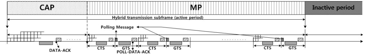
**Fig. 1** Mixed Period (MP): A CAP slot (CTS) is inserted in front of each GTS for immediate transmission of emergent data.
