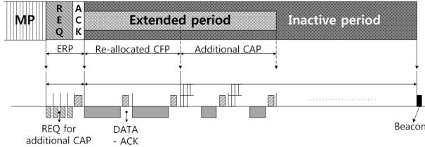
**Fig. 3** Extended Period (EP): Re-allocated CFP and additional CAP can be used in inactive period, if needed.
