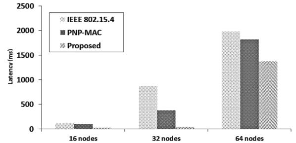
**Fig. 4** Medical traffic (BO=4/SO=3): Due to priority-based CTS and re-allocated CFP in EP, the proposed scheme provides the lowest latency for medical traffics.
