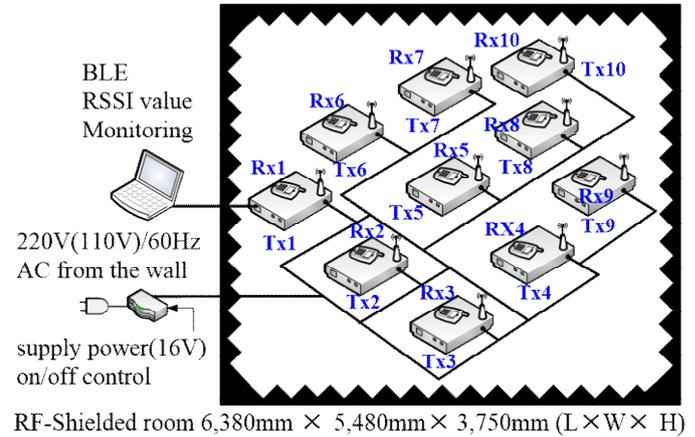
Fig. 3 Diagram of the CCA technology test set for 10 wireless charging pads (Tx's) with single Rx each in a dense environment
