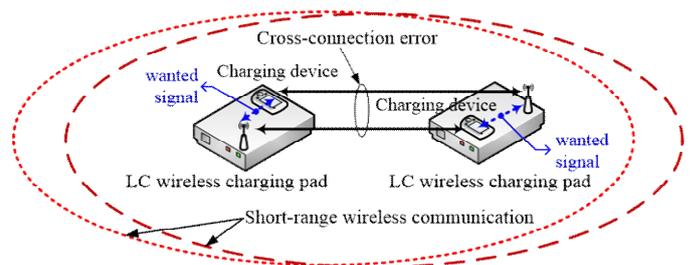
Fig. 1 Cross-connection errors occur between the wireless charging pads (Tx) and charging devices (Rx) within the same wireless communication range.
