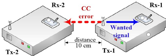
**Fig. 5** Schematic diagram of the test set in a closely located LC wireless charging pad environment. Rx-1 is belongs to Tx-1, whereas Rx-2 is cross-connected.
