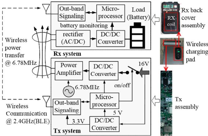
Fig. 2 Block diagram of the LC wireless charging system
