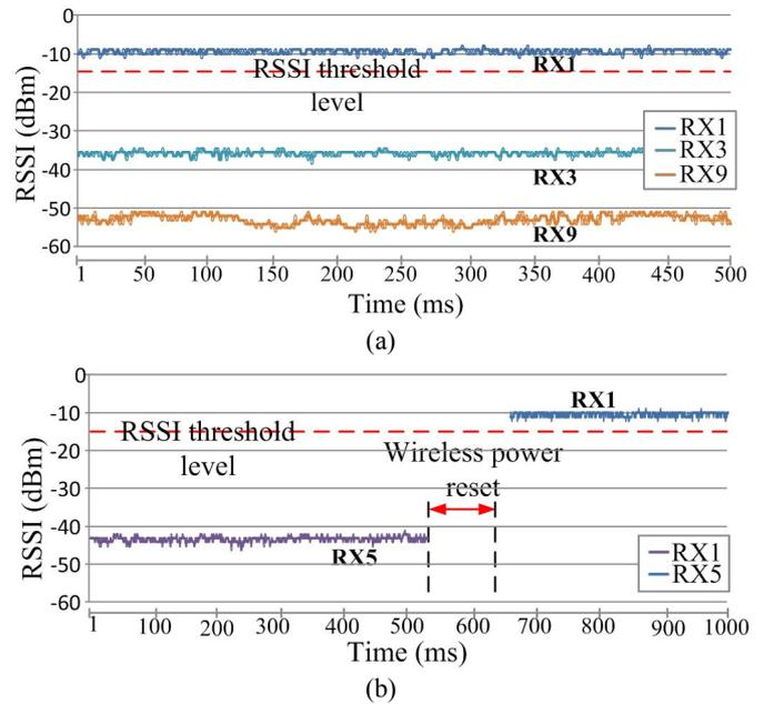
Fig. 4 Measured RSSI values for the proposed CCA technology. (a) Normal RSSI detection of Rx's when Tx1 is the base pad. (b) RSSI values of reconnected Rx1 after wireless power reset control.
