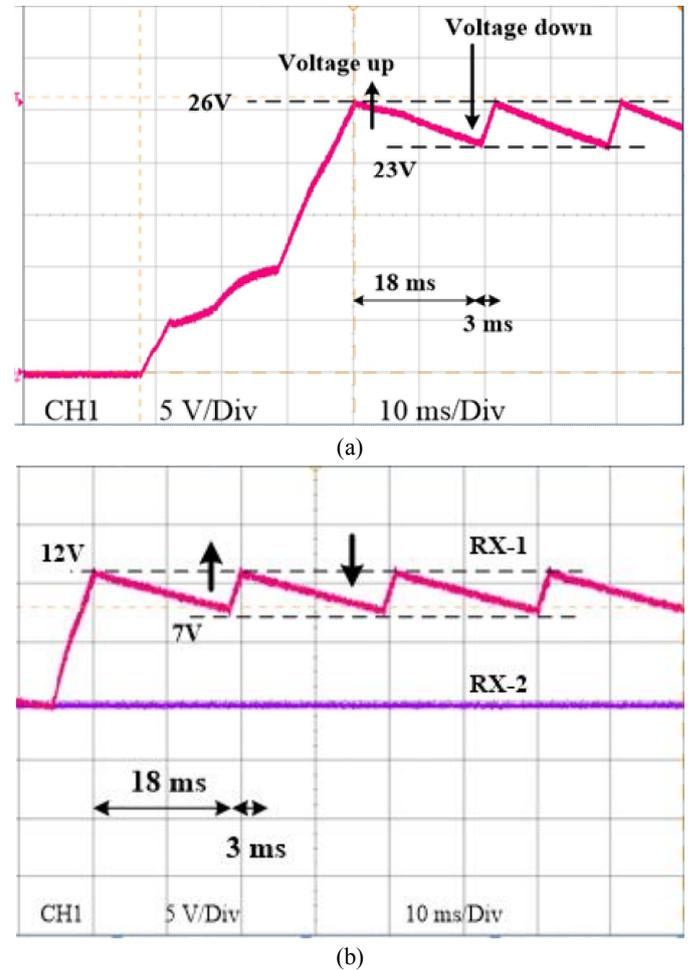
**Fig. 6** Measured voltage waveforms in a Tx and Rx's shown in Fig. 5. (a) Output voltage waveform of the power amplifier in Tx-1. (b) Received voltage waveform at Rx-1 and Rx-2.
